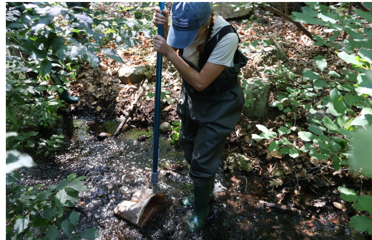
Collecting benthic macroinvertebrates using the kick net sampling method in Muddy River (CRWA)
